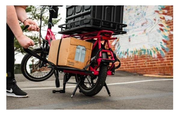
Since the bike industry lacks an official kickstand standard, Tern worked with EFBE, a leading German testing laboratory, to develop a custom kickstand test for the Lockstand QuadStruts. The kickstand passes 30,000 engage/disengage cycles with a load of 100 kg, which would approximate 3 years of hard, daily, commercial usage at max loading.
