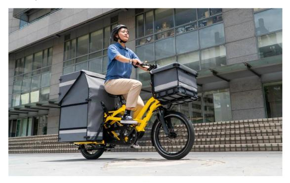
The Cargo Box 300 is designed for the GSD and has a capacity of approximately 300 liters. It is designed for heavy cargo and packages, with internal shelving that helps organize the interior space for parcels of different sizes. The Cargo Box 37 measures  $30 \times 40$  cm and is designed for the Transporteur Rack, which can be fitted to the front of any of Tern's cargo bikes.
