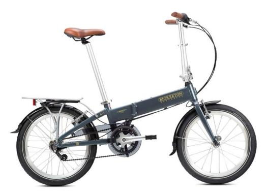
Argent 1707 City – Bickerton has been asked for hub gears on the Argent... Here it is... with Shimano Nexus 7 speed priced at €799.
