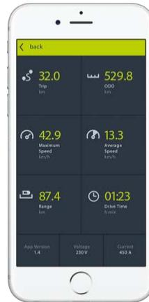
Ride mode shows key data such as trip and total distance, maximum and average speed, plus range remaining.
