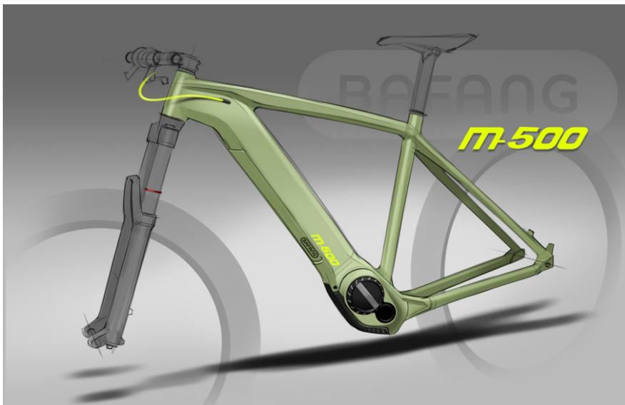
Bafang M500 center motor with integrated downtube battery in a FS and Hardtail frame concept
