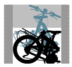
The Vektron is a 250W-Bosch ebike that you can take anywhere. It folds in under 10 seconds to the smallest size of any bike in Tern's lineup (86 x 68 x 36 cm, 21.8 kg), while delivering all the ride quality of a full-sized Bosch e-bike. When
