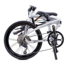
Tern's new Verge bikes begin with 451 mm (22") wheels, which offer 10% higher gearing than 406 mm wheels. That means the bikes achieve downhill gearing — up to 102 gear inches on the Verge X11 — using standard equipment.
