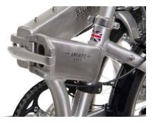
As Mark Bickerton explains: "The elegant hinge assembly has a very low profile design. For strength and a long life span, it uses integrated bearings and stainless steel pivot pins giving smooth folding and easy serviceability. The lightweight interlocking three dimensional structure of the hinge abutment prevents torsional movement better than any other folding bike hinge. With a secondary safety lock and a high-
