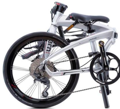
Tern’s new Verge bikes begin with 451 mm (22”) wheels, which offer 10% higher gearing than 406 mm wheels. That means the bikes achieve downhill gearing – up to 102 gear inches on the Verge X11 – using standard equipment.
